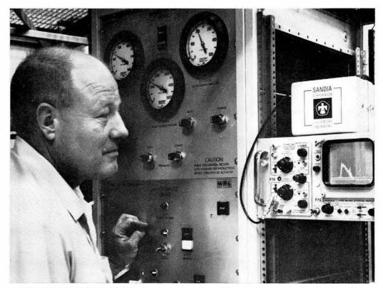
INITIAL-PEAK SAWTOOTH PULSE appears on the oscilloscope screen at the shock testing machine console, operated by A. W. Clark, Environmental Test Division I, 8112.
